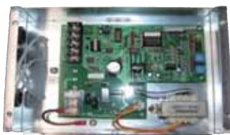
Modbus® Interface TCB-IFMB641TLE
